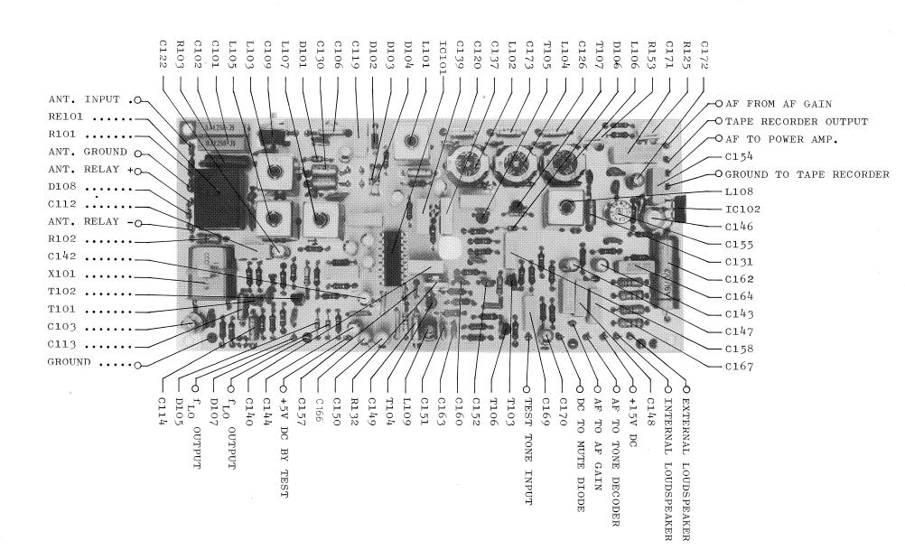
This printed circuit board contains the digital signal handling part of the receiver.
