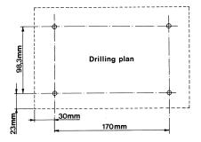
For mounting, dismantle the four screws on the front plate and disconnect the power and coaxial plug placed inside the cabinet. The four holes seen at the bottum of the cabinet should be used for mounting the cabinet on the bulkhead, ceiling or panel.
